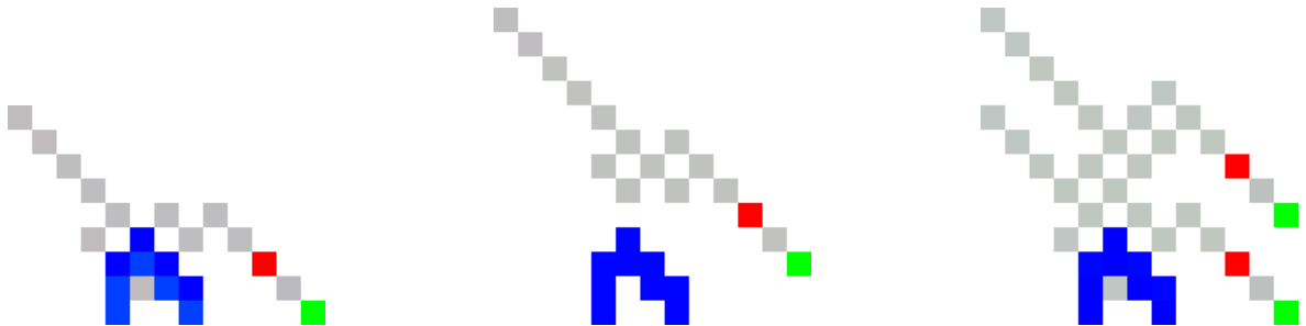
FIG. 10. Three cases in the operation of a switch gate. Left: A = 0, B = 1 . Center: A = 1, B = 0 . Right: A = 1, B = 1 . Particles are heavily shaded, cluster is black, and paths are lightly shaded. The path shading is only for every alternate time step, to make it simpler to resolve distinct paths by eye. The null case, A = 0, B = 0 is omitted.
